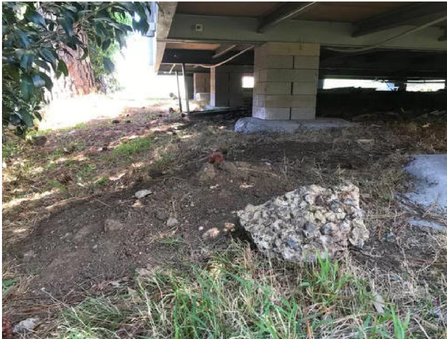
Photograph 9; evidence of demolition rubble and anthropogenic materials on the ground surface in a suspected fill area
